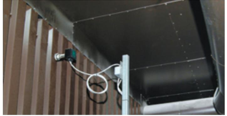
Electrodynamic sensor mounted in chamber wall
