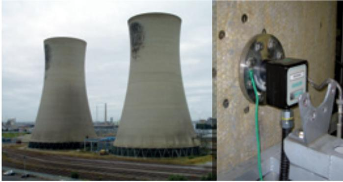
Approved (MCERTS /TUV) Dynamic Opacity Instruments monitoring the output from a Boiler Plant Electro filter on a Coal-Fired Power Plant
