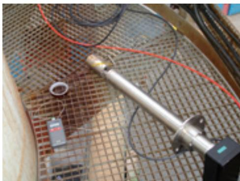
Pro-Scatter sensor incorporates a moveable flange to allow appropriate insertion into the gas steam
