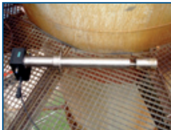
Pro-Scatter and Electrodynamic Main Stack Sensors
