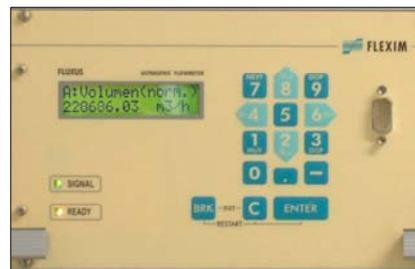
The integrated flow calculator of the transmitter makes it possible to process external temperature and pressure measurements, and to convert the measured actual volumetric flow to standard volume/mass flow.
